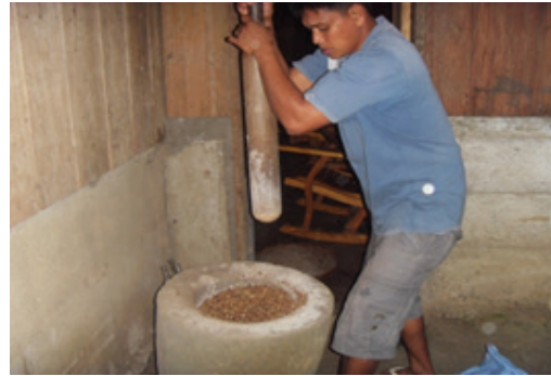
Figure 8. Dehulling using pounding method
