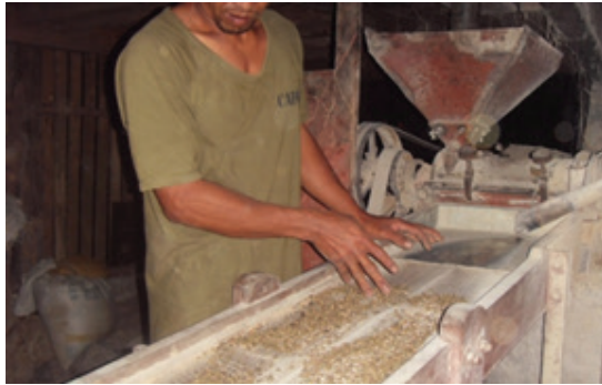
Figure 7. Dehulling using mechanized dehuller.
